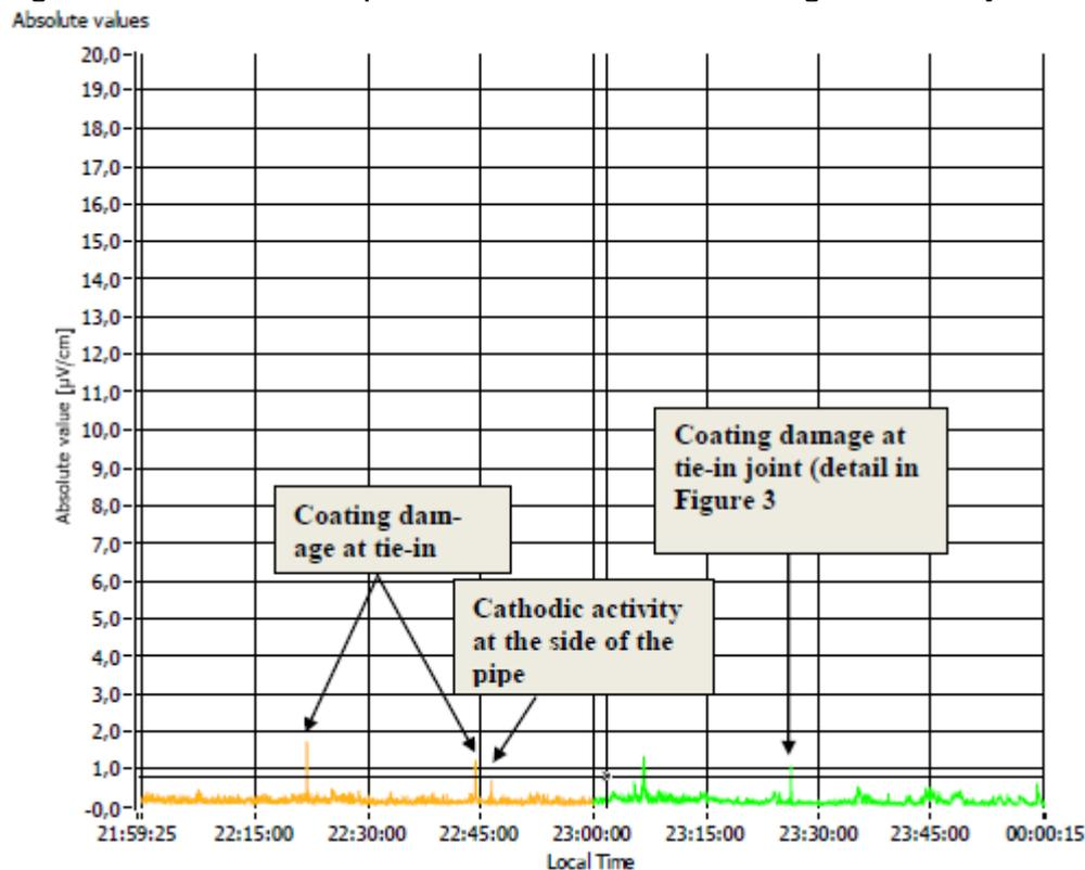
**Figure 2:** Field gradient absolute values along a 2 km section of pipeline, measured between 0.5 and 1 meter above TOP. These are unfiltered RAW data measurements. [7]
