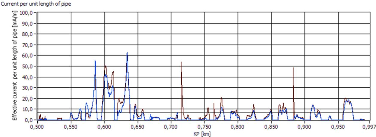
Figure 5. FG data from two sensors given as effective current per unit length of bundle
