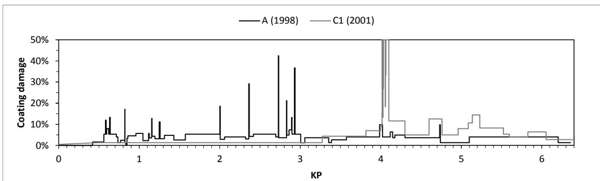
Figure 3. Coating damage as percentage of bundle circumference vs. kilometre point (KP) (2013)
