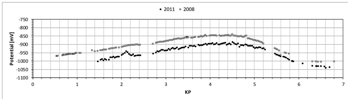
Figure 4. CP stab potential profile for bundle C1 in 2011 and 2008
