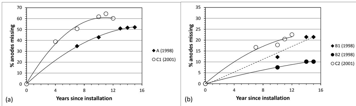
Figure 2. Percentage anodes missing: (a) extensive impact of trawling and (b) less impact of trawling
