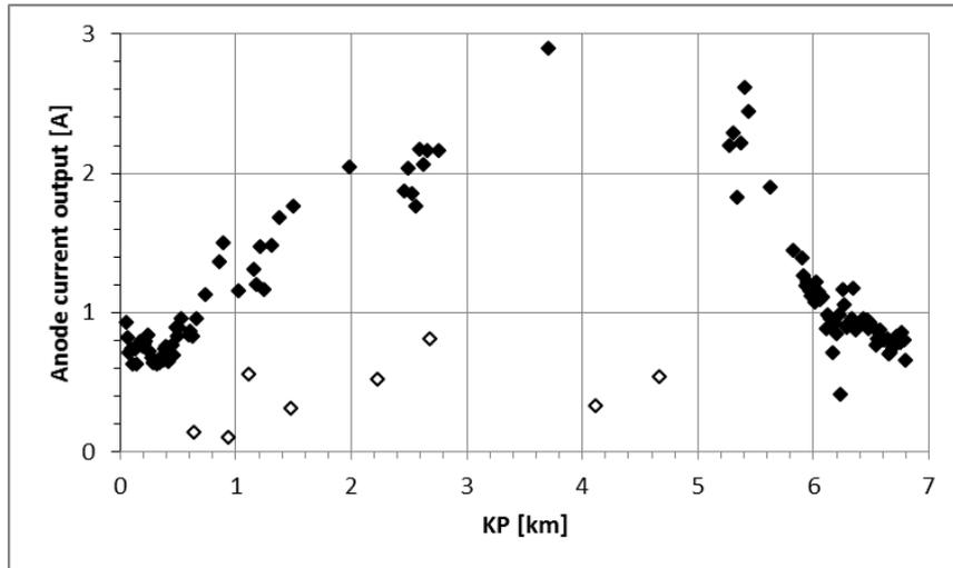
Figure 7. Current output from remaining bracelet anodes on bundle C1: Intact anodes (closed symbols) and damaged anodes (open symbols)
