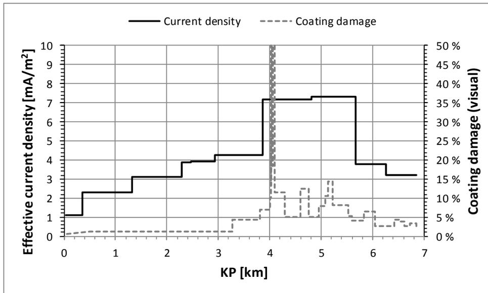
Figure 6. Effective cathodic current density and visually determined coating damage for bundle C1
